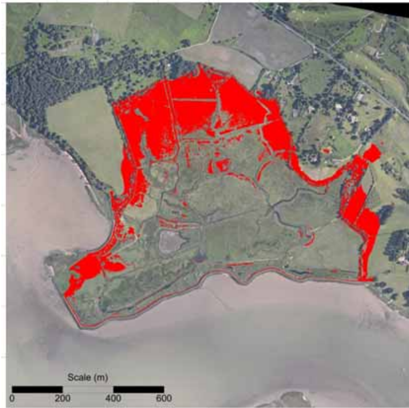
Figure 32. The potential saltmarsh elevation 'window' (between 0.9 and 1.7 m OD), highlighted in red, on Hazlewood Marshes
