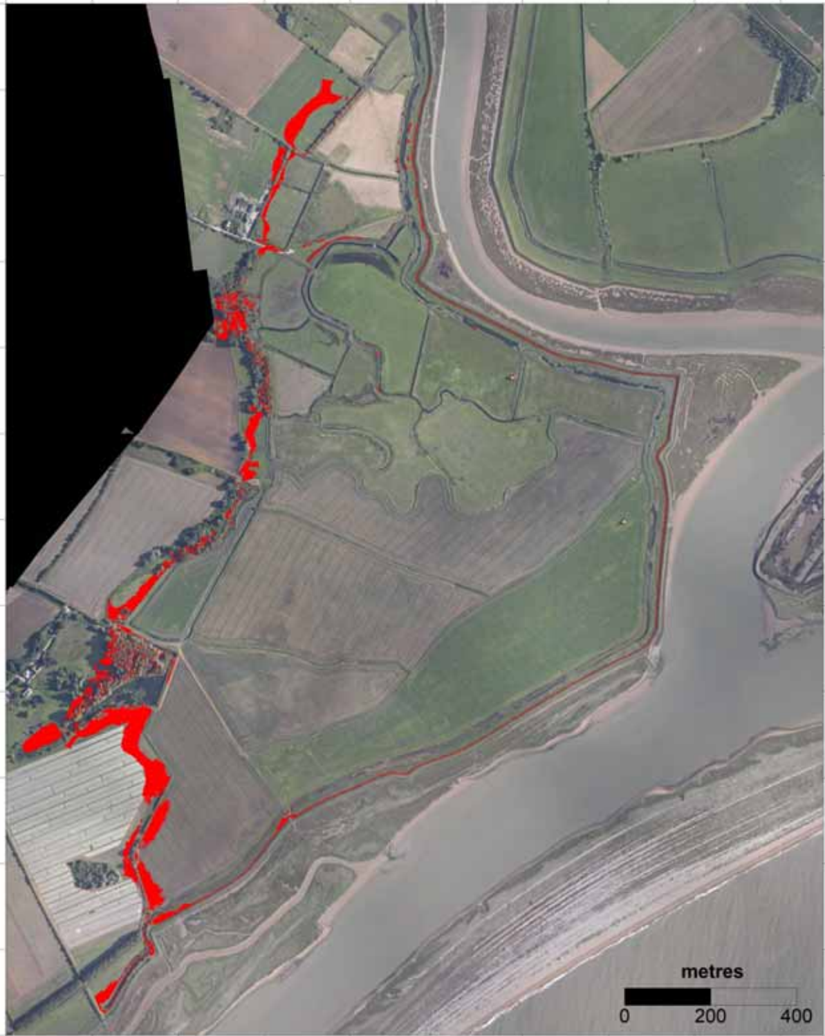
Figure 41. The present saltmarsh elevation 'window' on Boyton Marshes area between 1.0 m OD (MHWN) and 1.53 m OD (HAT), highlighted in red
