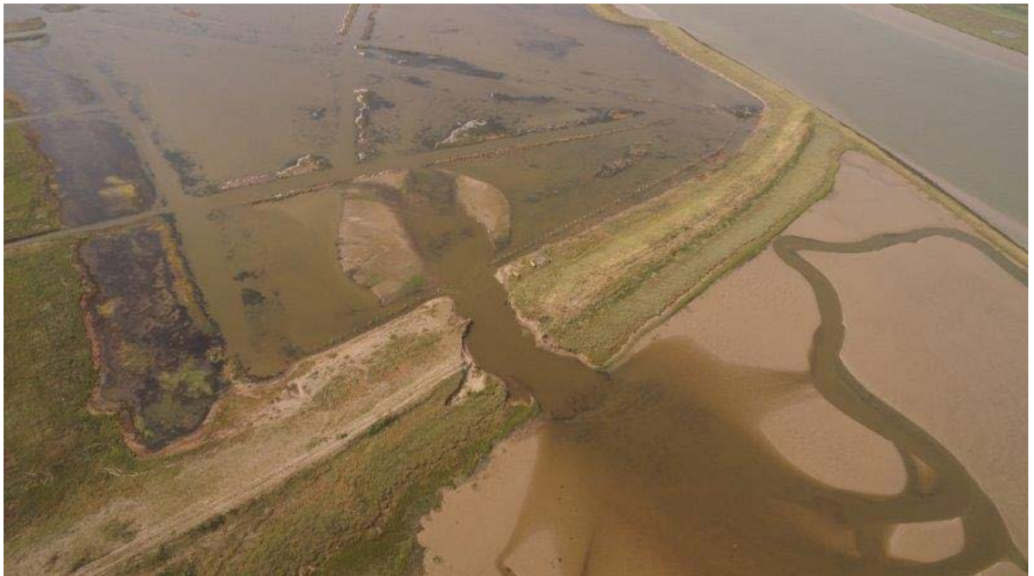
The result of the 2013 tidal surge on the American Wall, which has now been repaired. Photograph by Andrew Hawes.
